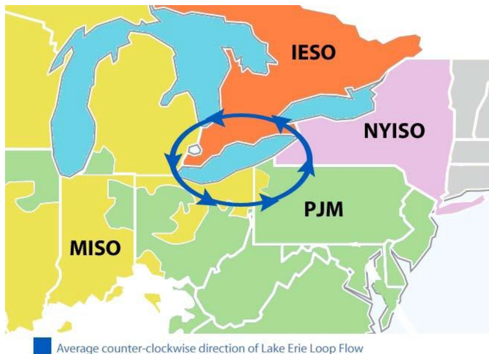
Figure 7: Average Flow of Electricity around Lake Erie. Electricity generally flows as shown in Figure 1 but this can change depending on the physical operating conditions
