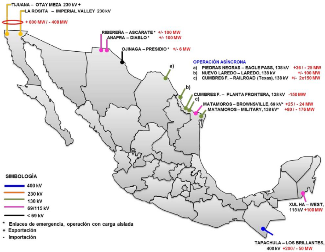
Figure 38: Cross-Border transmission lines to Mexico, 2014. No 400 kV lines interconnect the United States and Mexico; larger (synchronous) interconnections exist between California and Baja California, while intermediate, asynchronous connections exist between Mexico and Texas. Two emergency 69/115 kV lines interconnect Mexico and New Mexico. (International Energy Agency, 2016)
